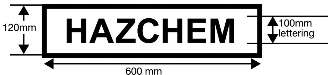
13.1 Form and dimensions of outer warning placard
