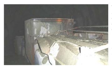
The photo shows the rear view of the bogger that was removing the wet cuttings from the base of the raisebore hole at the time of the inrush.
