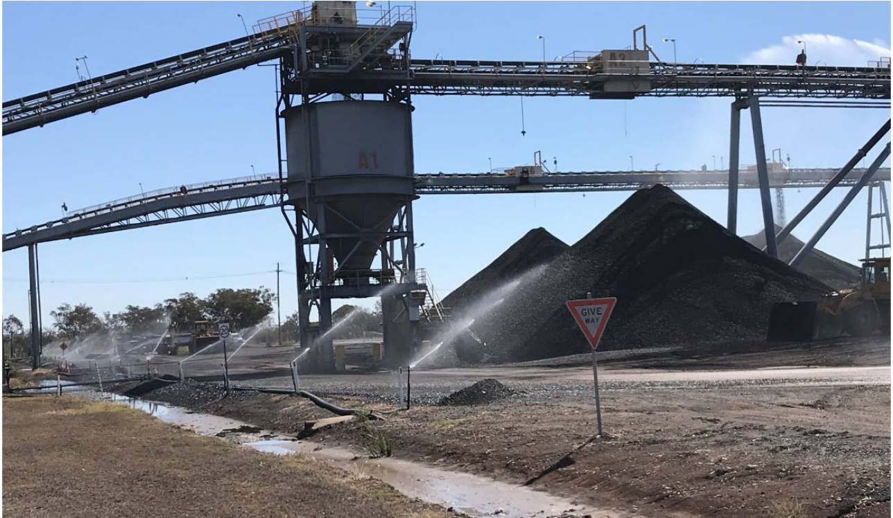
Figure 12. Sprinklers suppressing dust on roadways
