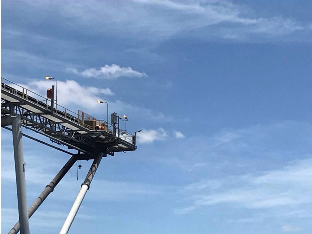
Figure 3. Cannon on conveyor delivery points to suppress stockpile dust
