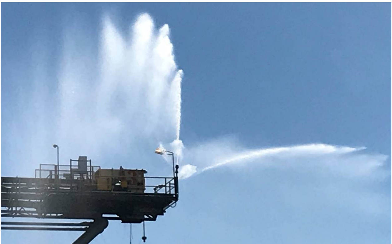
Figure 4. Cannons on conveyor delivery points to suppress stockpile dust
