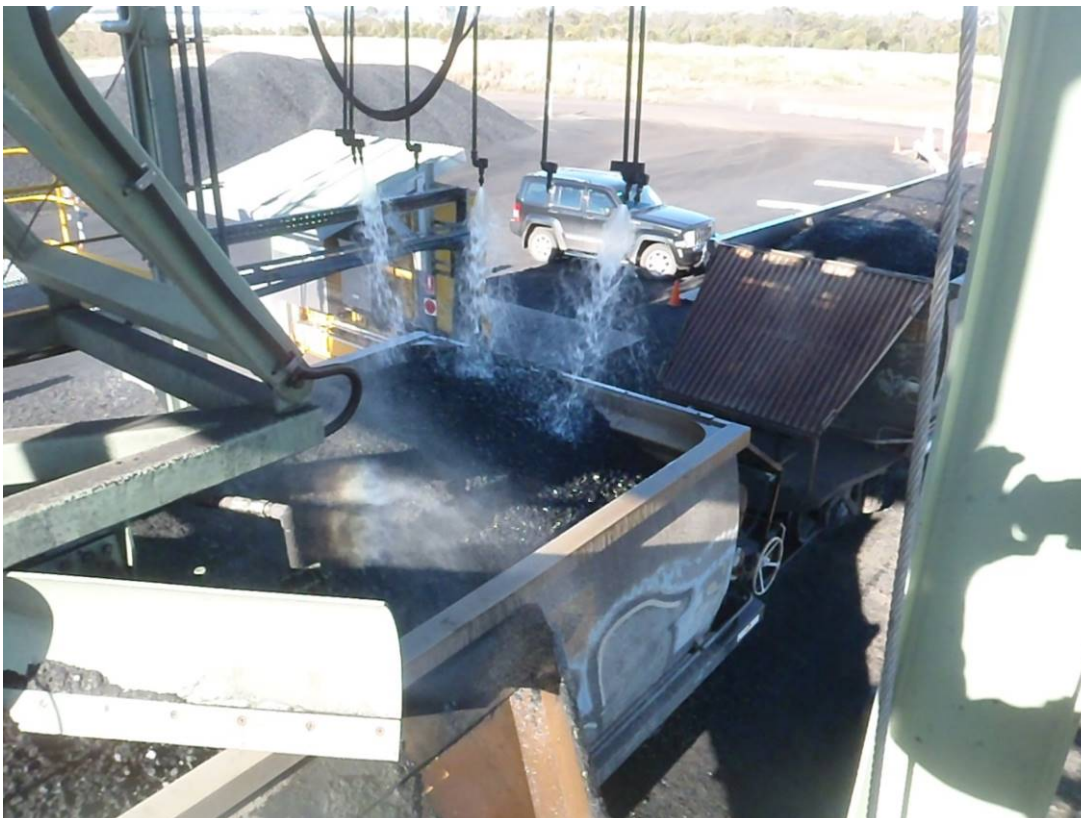
Figure 17. Profiler and Veneering Solution being applied
